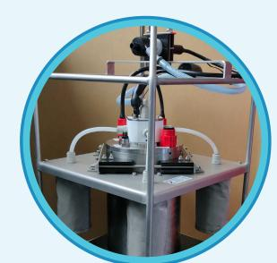
Submersible Sampler for Nanoplastics and Microplastics – SuNaMips
