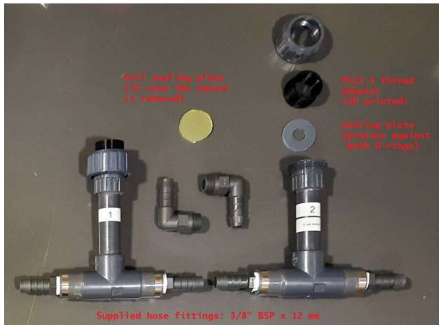
Figure 62: Versions of the cuvette that have been produced. Cuvette nr. 2 has been made about 2 mm shorter than nr. 1, in case it is found that the sensor needs to be slightly deeper inside.
