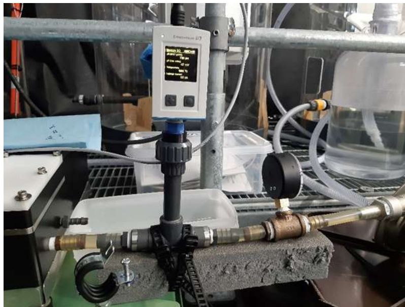
Figure 63: The sensor, its transceiver and cuvette being tested in series with AFT-pH sensor.
