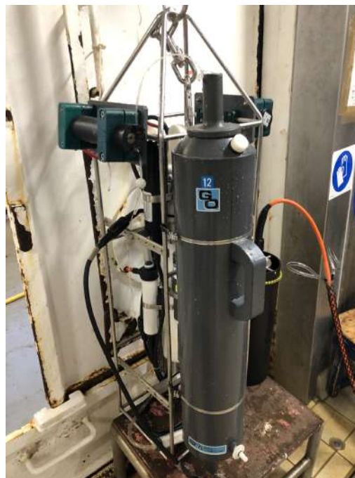
Figure 4: CTD, sampling bottle, DO and Chl- a prototypes mounted on a frame used to perform water sampling and simultaneous profiling during the IBTS cruise.
