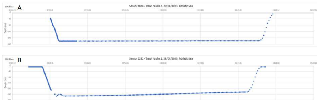
Figure 43: Depth profile recorded by the prototypes during the fishing tests. A) depth profile acquired by prototype 8888 during a fishing operation in which the fishing depth was reached before the change in data acquisition settings, B) depth profile acquired by prototype 2222 during a fishing operation in which the fishing depth was reached before the change in data acquisition settings.
