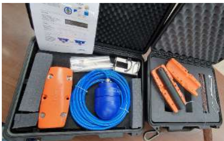
Figure 31: NKE equipment received by CNR: DO and Chl- a prototypes, plastic sensor protections, WiHub receiver, relative accessories for mounting and connection and quick start guide.
