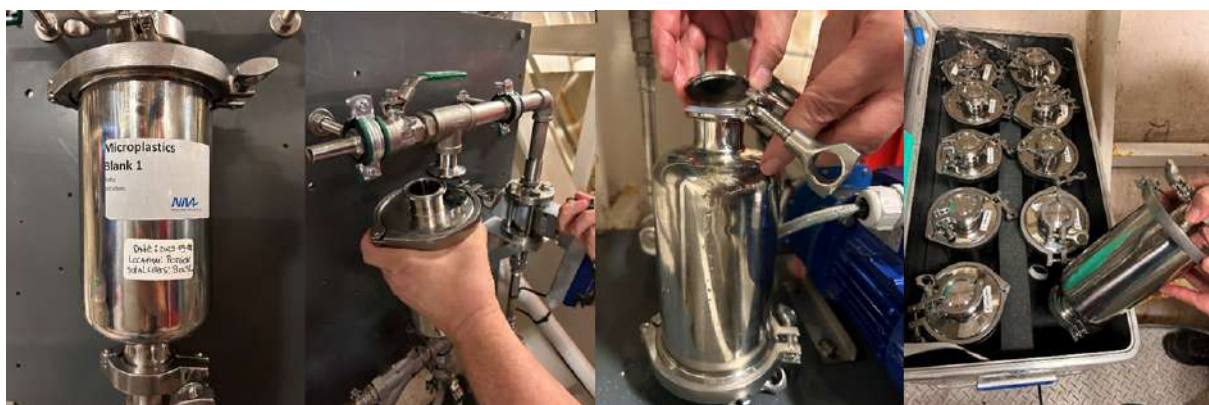
Figure 75: The filter unit and replacement of the whole filter unit to avoid contamination.
