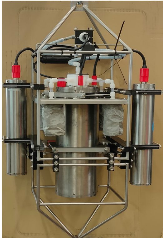
Figure 25: The SuNaMiPS with external batteries attached - ready for deployment.
