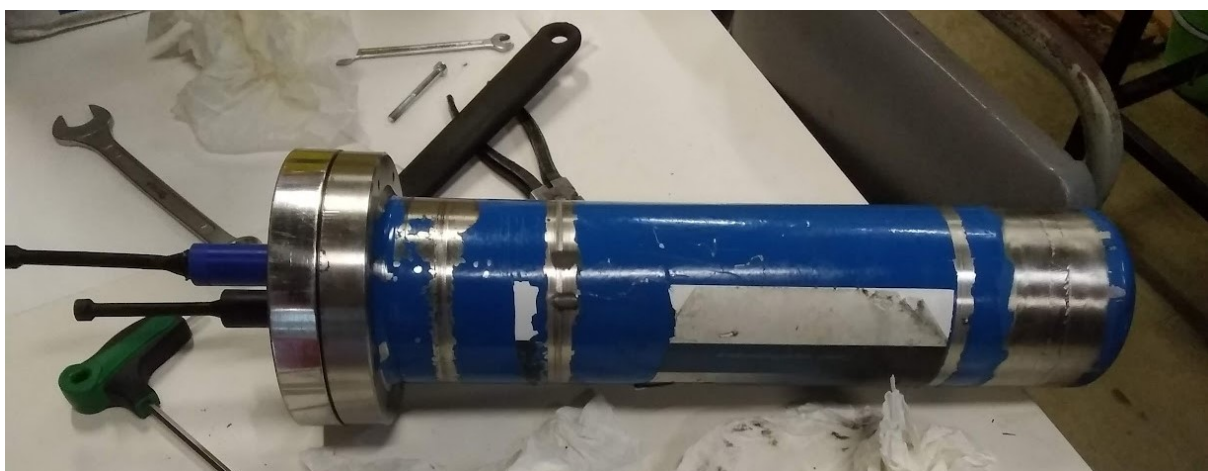
Figure 33: Deep-ocean low-level radioactivity sensor.
