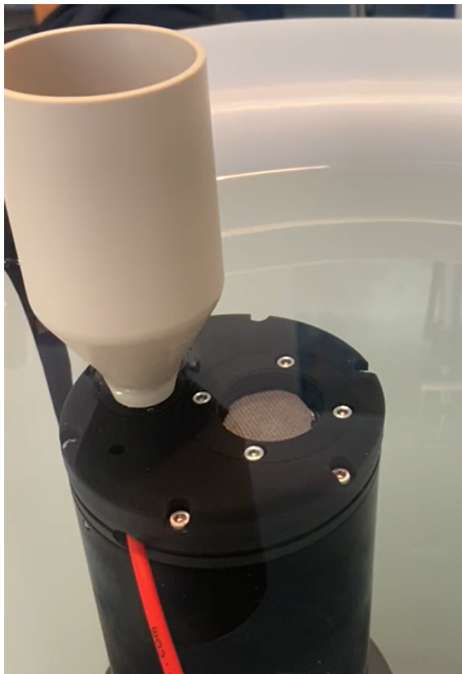
Figure 8: Silicate sensor equipped with funnel for laboratory experiments immersed in artificial seawater tank.
