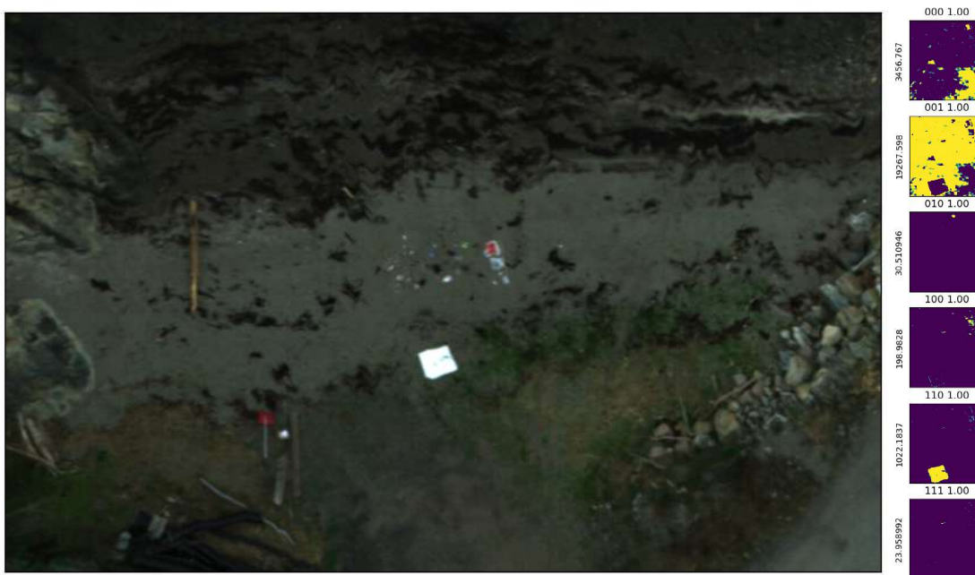
Figure 18. Left: AFX10 hyperspectral camera RGB image over the beach (bright white object if the reference target).
