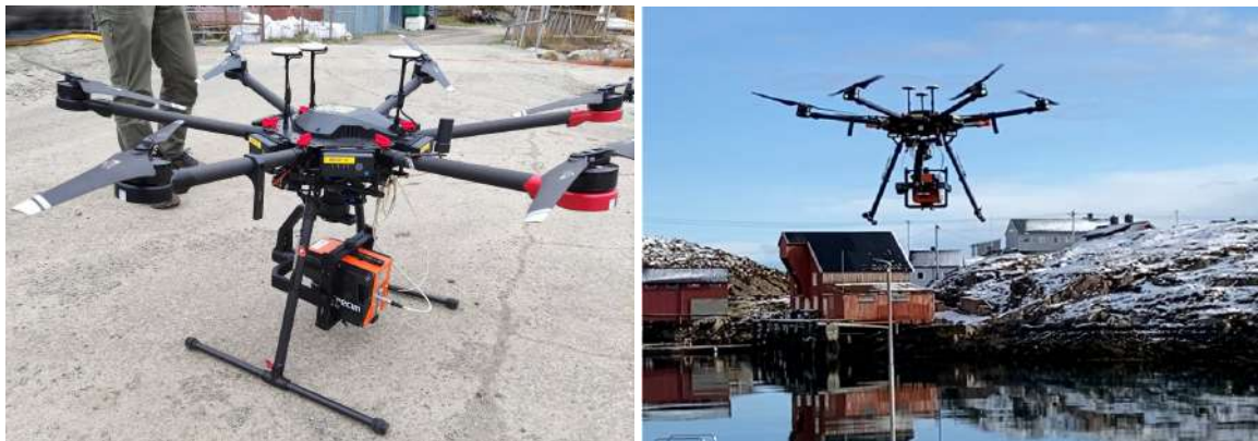
Figure 6. UAV 1 – Hyperspectral imager: DJI Matrice 600 Pro, with Specim AFX10 Hyperspectral camera.
