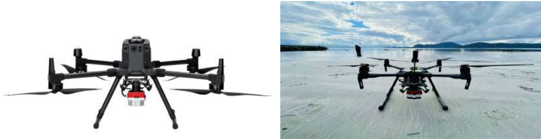
Figure 7. UAV 2 – Multispectral imager: DJI Matrice 300 RTK, with Micasense ALTUM PT.
