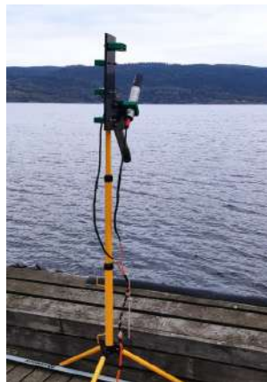
Figure 2. Downwelling Irradiance Sensor mounted alongside the RAMSES radiometer.
