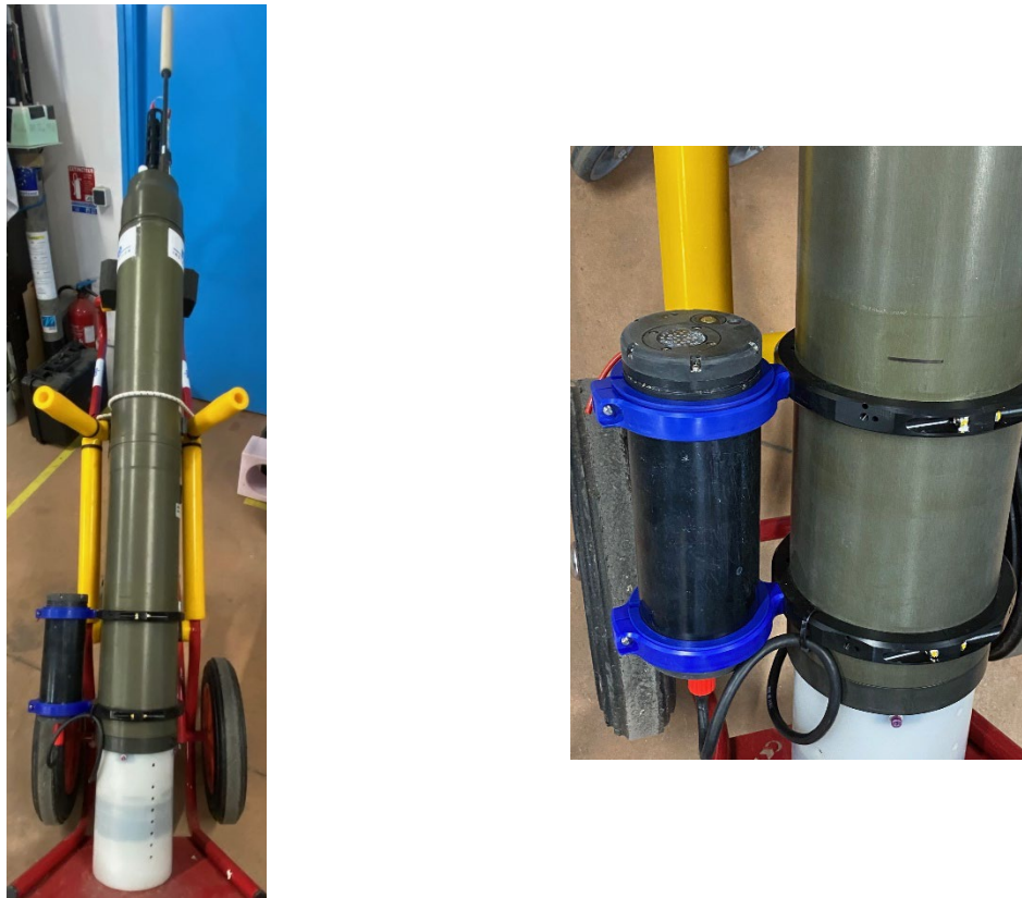
Figure 20: Final integration of silicate sensor on a CTSS float
