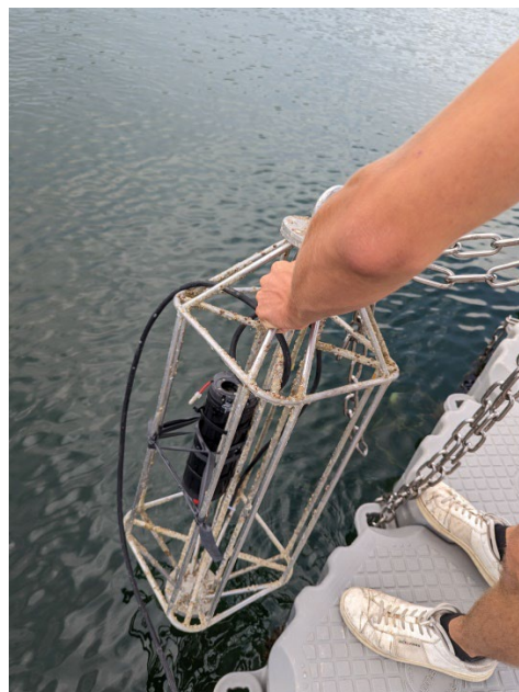
Figure 15: A silicate sensor (autonomous version) mounted on a rosette for field validation
