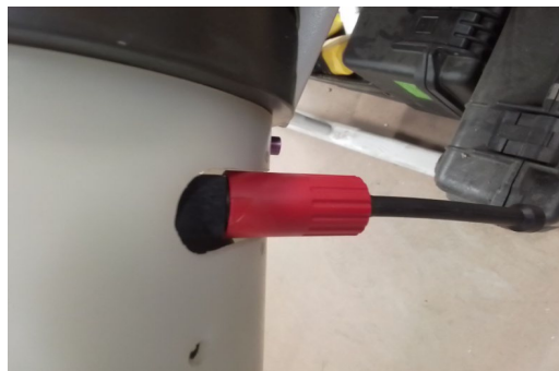
Figure 10: Subconn connector on the float side
