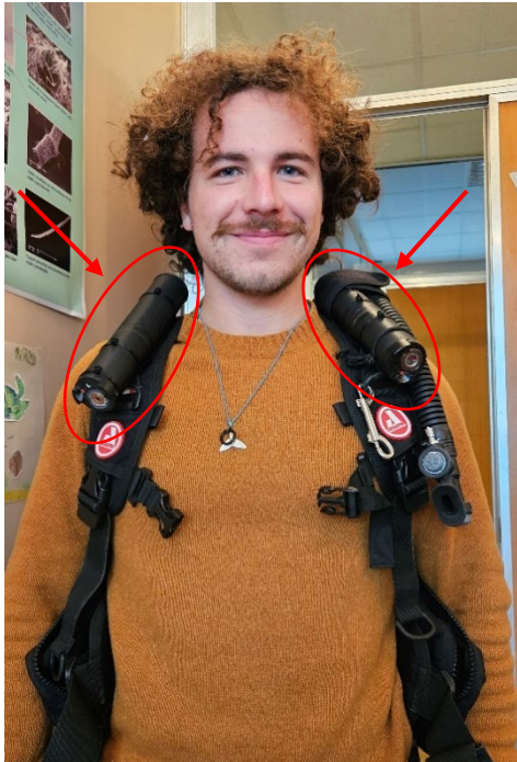
Figure 21. Positioning of WiSens DO and Chl-a sensors (red circles and arrows) on the BCD jacket of the divers.
