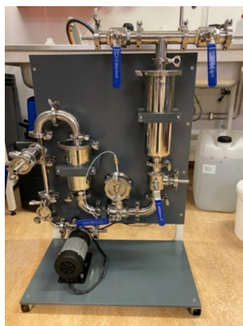
Figure 21: The standalone prototype of the combined sampler and oxidation and Nile Red dyeing chamber.
