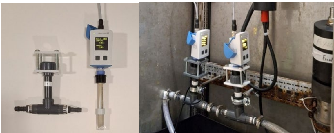
Figure 23: Left: The custom cuvette and the sensor. Right: The sensors connected in series with the Ferrybox instruments. Photos Sami Kielosto.
