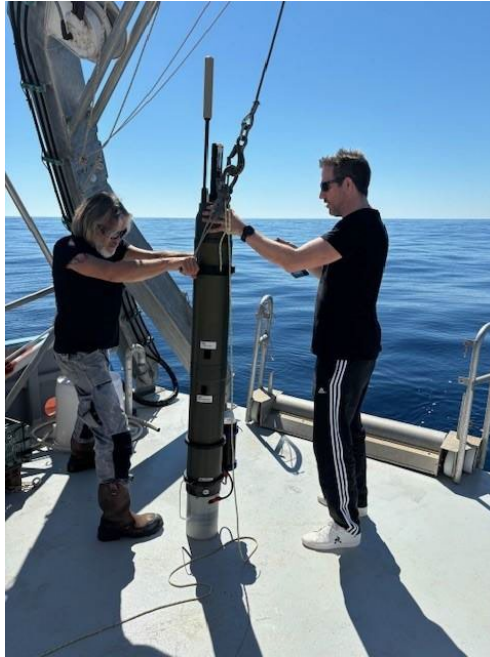
Figure 15: Silicate profiling float fixing system for launching
