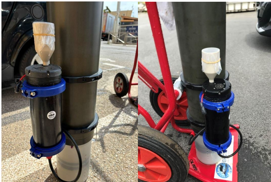
Figure 4: Integration of silicate sensor on the CTS5 float
