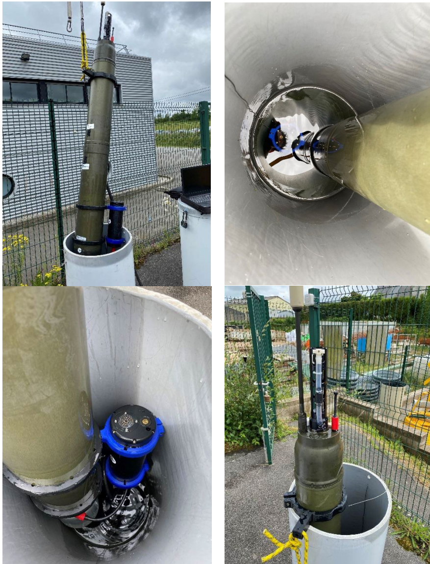
Figure 23: Tests of silicate probe in a freshwater tube (6m of depth)
